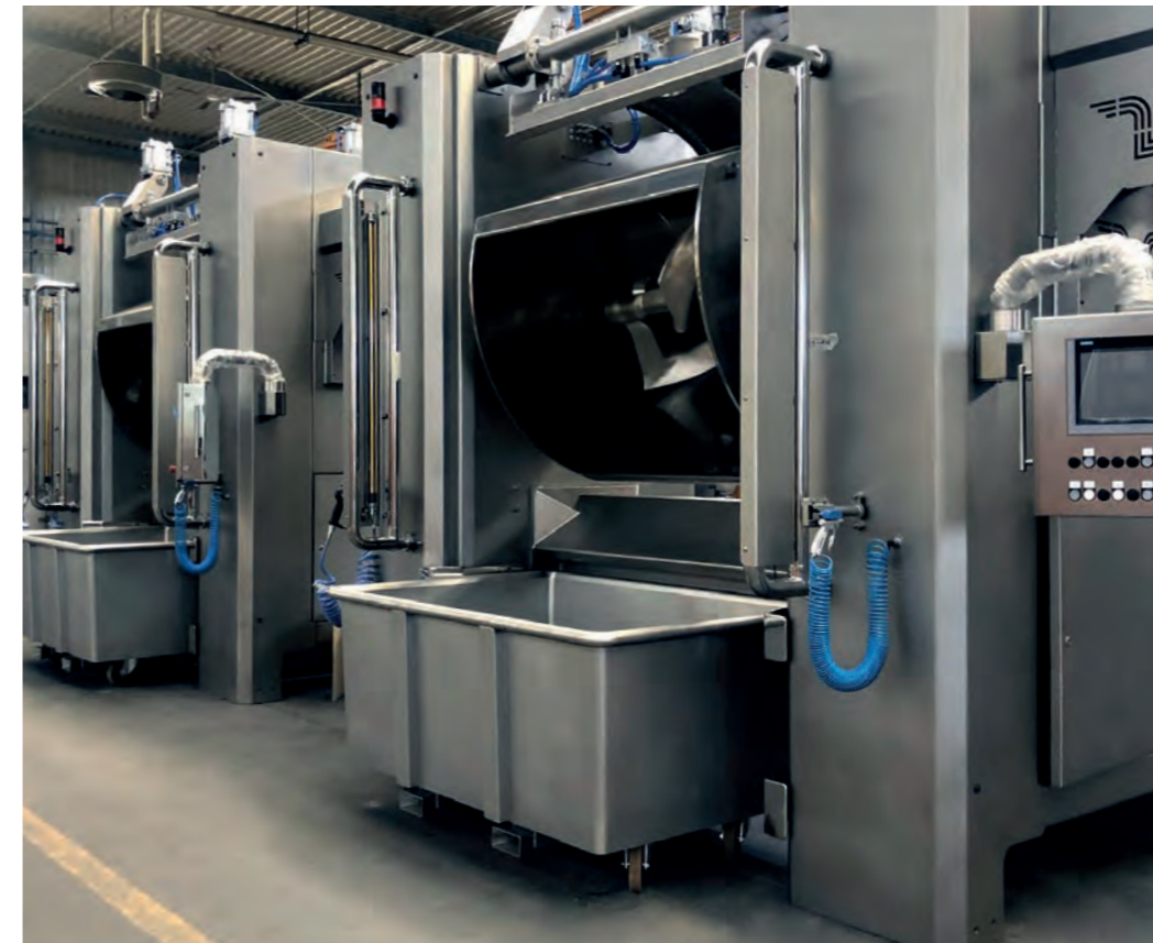
Horizontal mixing plant
