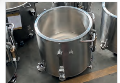
Detail of discharging valves for Multifunctional mixer
